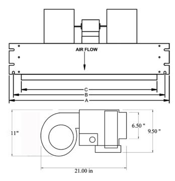
Copper stub out diameter: Suction: 3/4", Liquid: 3/8"
